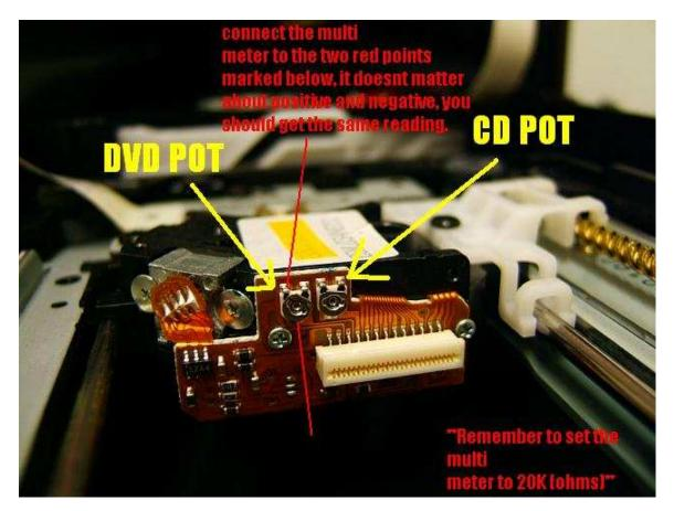
Now get your multimeter and set it to 20K (ohms). Connect it to the two connections on the pot. (doesn't matter about positive and negative, any way round will do) and take the reading.
