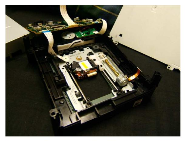
Now you should see the picture above. Remove the cable connecting the pcb to the lens so you have more room to calibrate the pot. Now look at the pic below.
