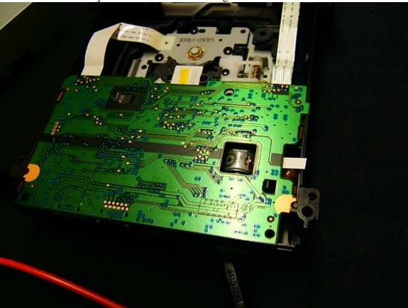
You need to push the black tab on the bottom right to one side, this lets you lift up the pcb. Do this VERY slowly as it will only lift up a little. One you have lifted it a tiny bit you can remove the cable which is holding the pcb. In place, one you have removed this
